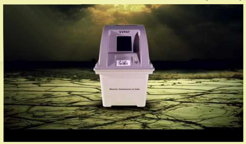
The VVPAT enables the voters to physically verify the vote cast on the EVM. It consists of the Printer Unit to print the voter's selection and the VSDU (VVPAT Status Display Unit) to display the error messages of VVPAT during poll.
